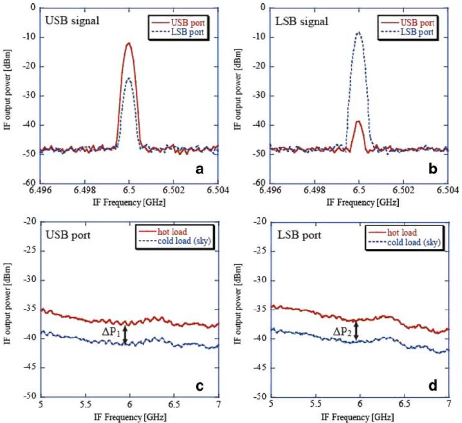
**Fig. 3** The IF power in the hot (bold line) and cold load (dashed line) of the USB (a) and LSB (b) shown as functions of the IF frequency. The difference in output power at USB is  $\Delta P_1$  and LSB is  $\Delta P_2$  when injecting the radiation of hot and cold loads. The IF power output of USB port (c) and LSB port (d) when injecting the test signal of USB (bold line) and LSB signal (dashed line).
