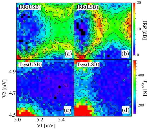
**Fig. 4** The IRR and  $T_{sys}$  of USB (a), (c) and LSB (b), (d) to combination of two SIS bias voltages.
