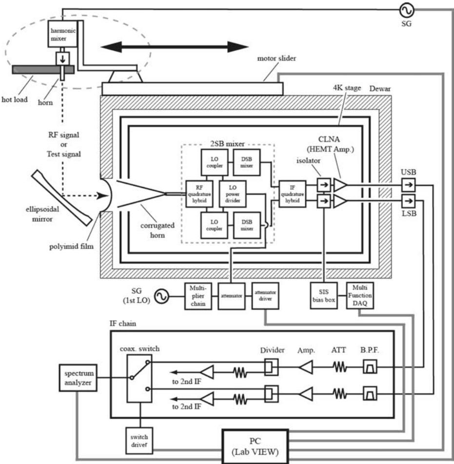
**Fig. 1** Block diagram of the 2SB receiver system. The figure shows the IRR measurement system, receiver dewar, and IF chain from above.
