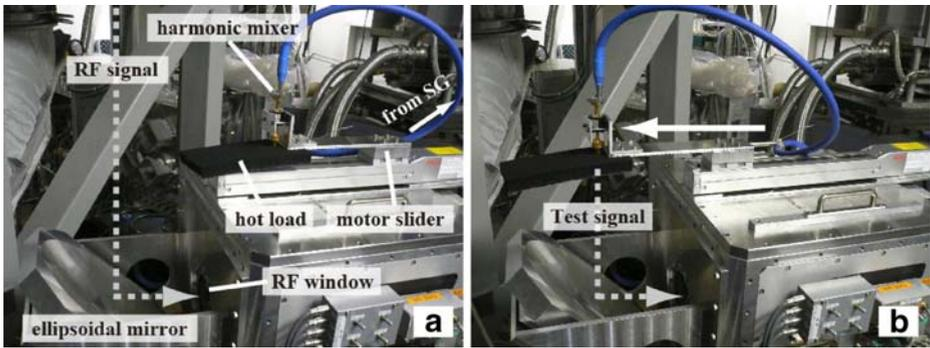
**Fig. 2** Photograph of the IRR measurement system on the top of the receiver dewar. It is located out of the beam from the main reflector during observations (a) and inserted in the beam center only at the measurement of IRR (b).
