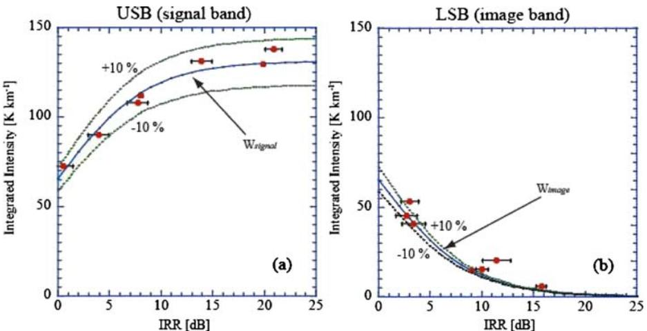
**Fig. 5** The relation between the IRR value measured by the IRR measurement system and the integrated intensity estimated from the molecular line observation in USB (a) and LSB (b), respectively. The bold line shows the anticipated value of the IRR according to the IRR calculation formula, and the dashed lines represent an error range of  $\pm 10\%$ .
